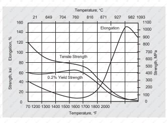
Figure 1. Elevated temperature tensile properties of annealed bar.
